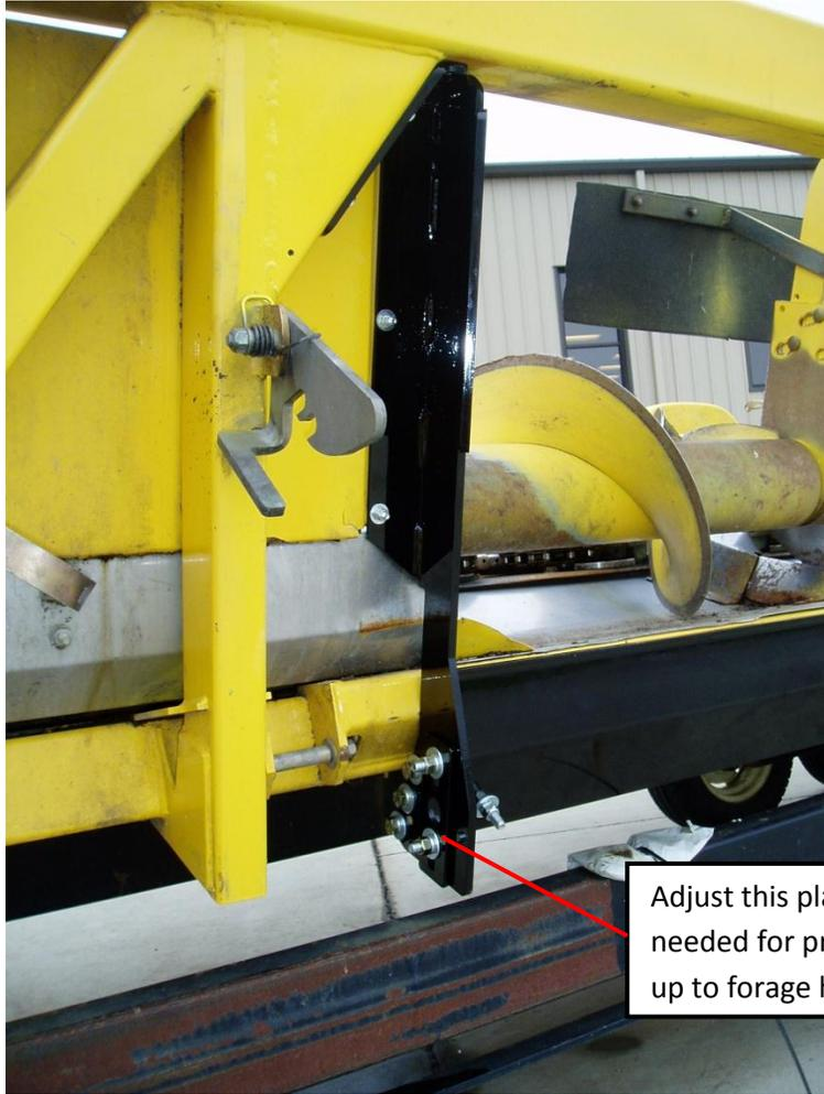
Adjust this plate as needed for proper fit-up to forage harvester
