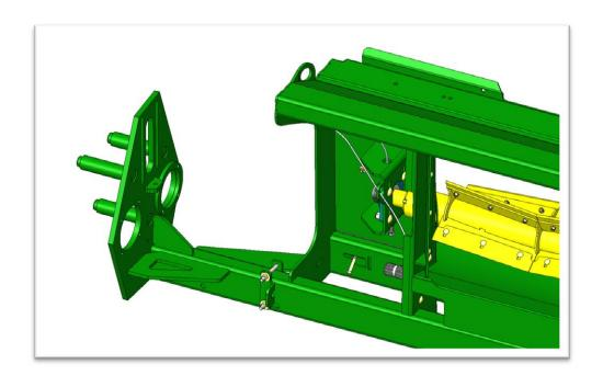
2) Cut off the large plate and gussets, so you are left with a bare tube and front gusset:
