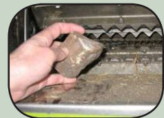
Disc wear after 190,000 tons of silage
