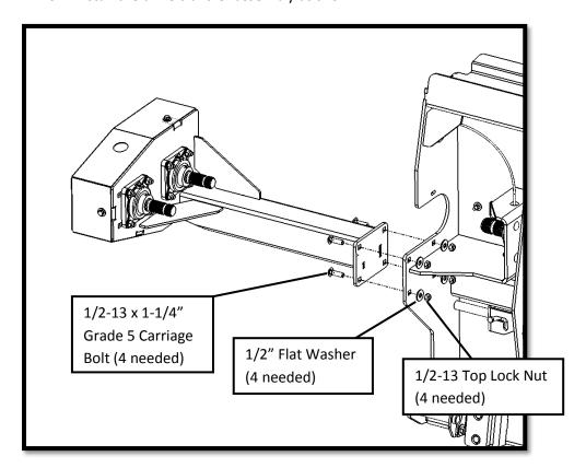
7. Install the PTO shaft as shown. The PTO shield is removed for drawing clarity, DO NOT REMOVE PTO GUARD.
