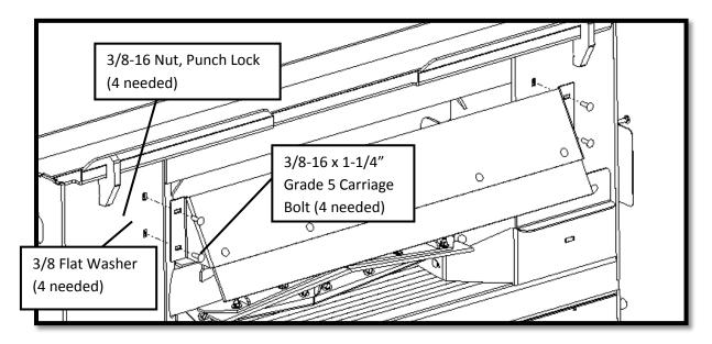
9. On your FX cutter, replace the front upper hanger bracket with the hanger bracket provided with the adapter. Be sure the Kooima bracket goes in the top three holes on the cutter.
