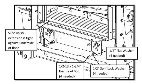
5. Install the spacer blocks and the latch pins as shown (left and right). Adjust the latch pin in/out to match the cutter after hanging adapter on the cutter for the first time.
