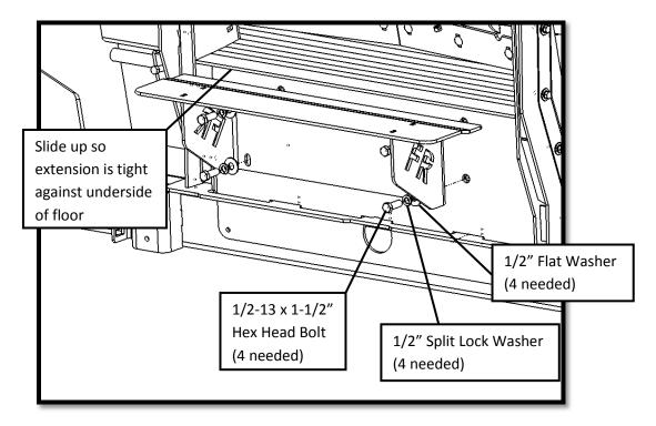
5. Install front shield as shown.
