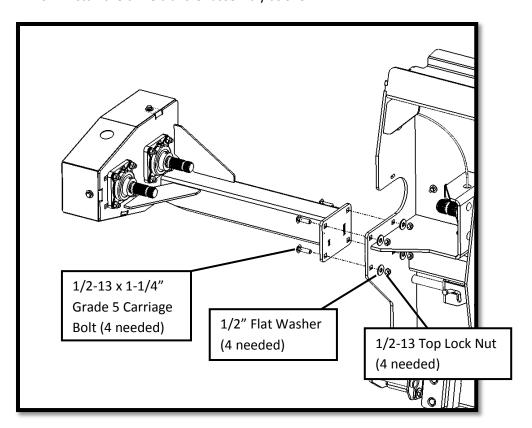
7. Install the PTO shaft as shown. The PTO shield is removed for drawing clarity, DO NOT REMOVE PTO GUARD.
